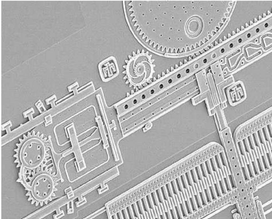
[ **Figure 2. Each of the basic elements of this electromechanical lock could be stored in a MEMS library to enable rapid reuse and design variations. Source: Sandia National Laboratories. ]**
