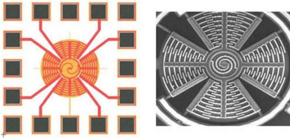
[ **Figure 4. Unlike IC layouts, which are rectilinear (Manhattan topology), MEMS devices have many curves and non-orthogonal angles. This makes the extraction task much more difficult. Newer field solver extraction tools, such as Mentor's Calibre xACT 3D, are key to addressing large, complex mixed MEMS-IC designs. ] Source: [http://jasonscarlett.com/\\_ucalgary/Gyro\\_Web/4.3.htm](http://jasonscarlett.com/_ucalgary/Gyro_Web/4.3.htm)**
